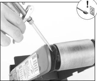
Figure 25. Lubricating the sleeve bearings.
